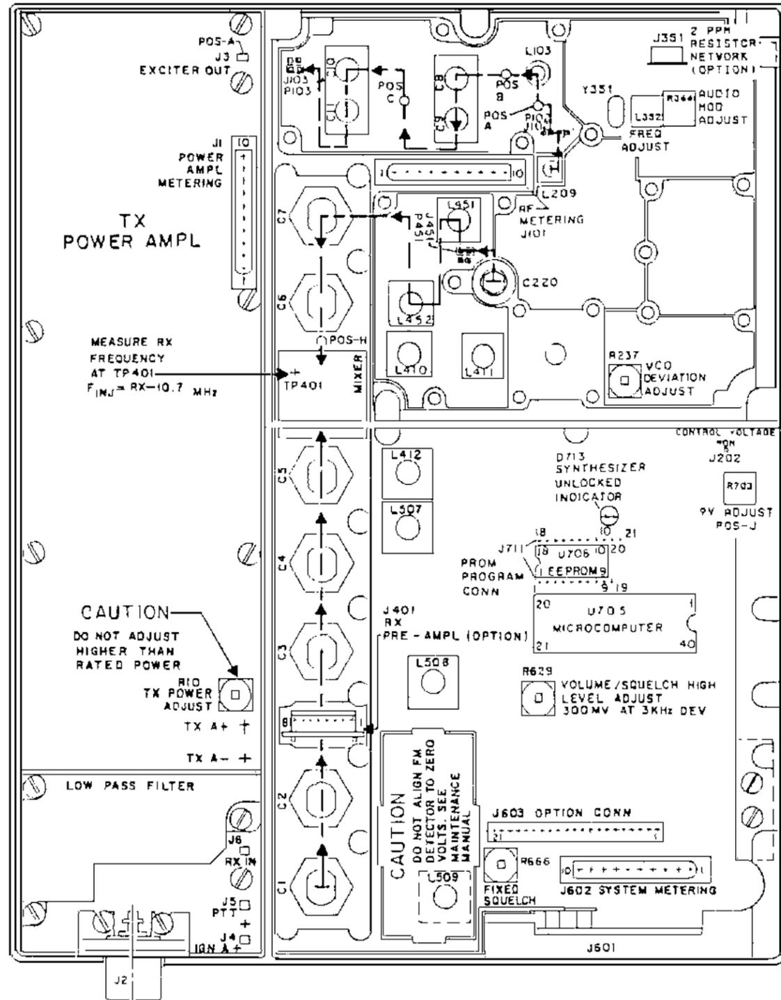
Figure 5 - Transmitter/Receiver Tuning & Adjustment Controls
