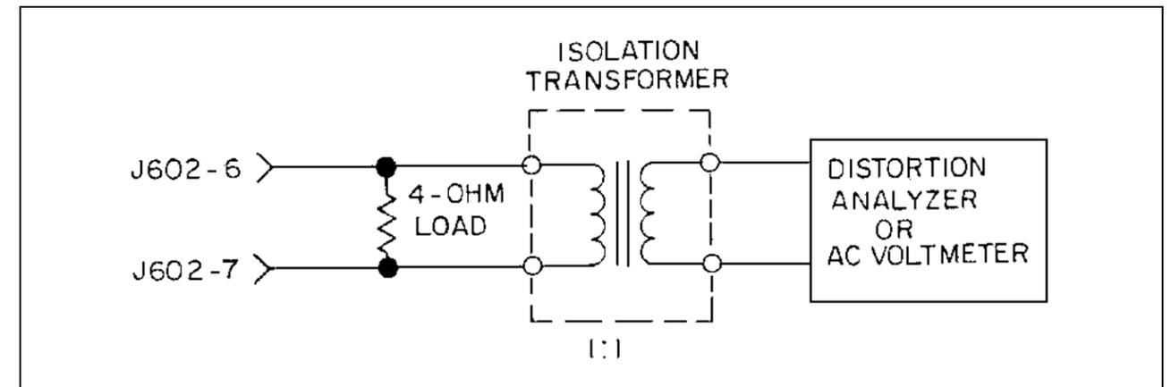
Figure 7 - Test Set-Up, Audio Output Measurement
